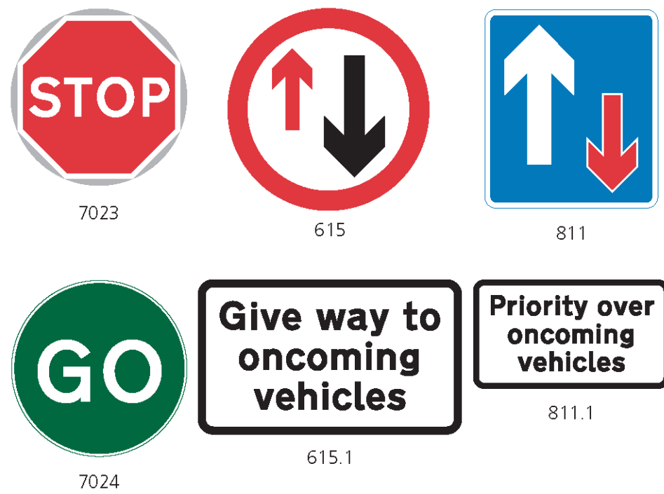
Figure 3.5: Manually Operated Stop/Go Signs and Priority Signs.
